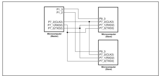
Figure 14.27 Serial Bus Communication Control Example (UART2)
